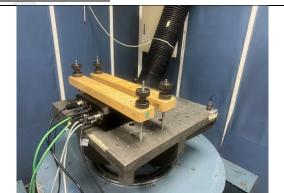
7. Vibration Test – Operating: Z axis
