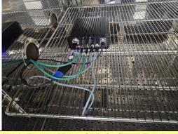
4. Damp Heat, Steady State Test/ Low Temperature Test – Operating
