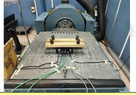
Vibration Test – Operating: Y axis
